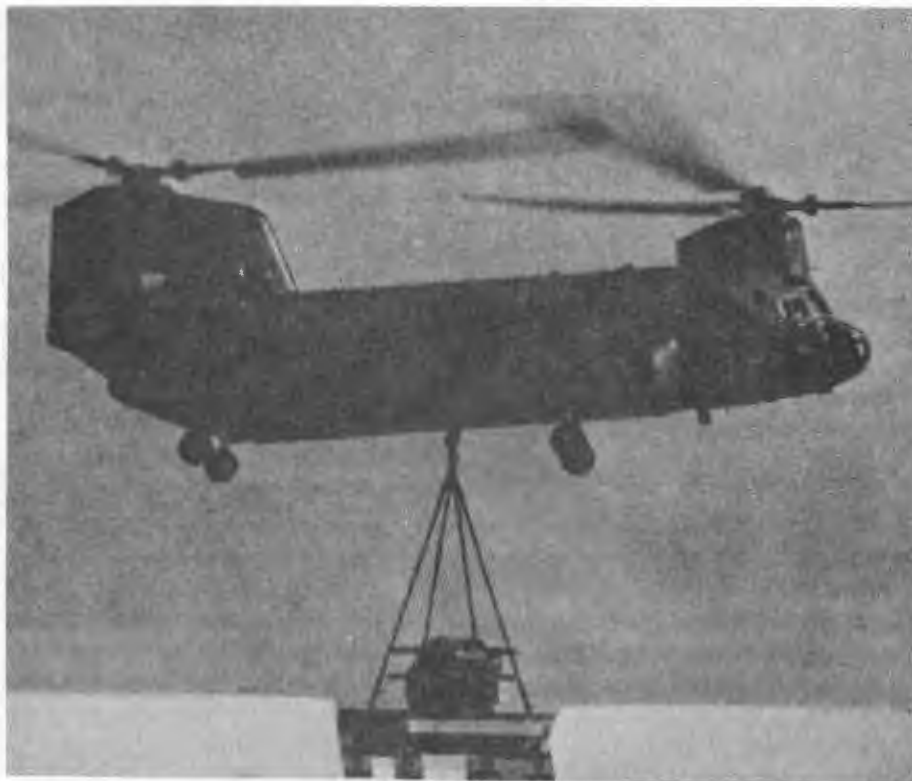
Figure 3-3. Airlifting launching station M54.
