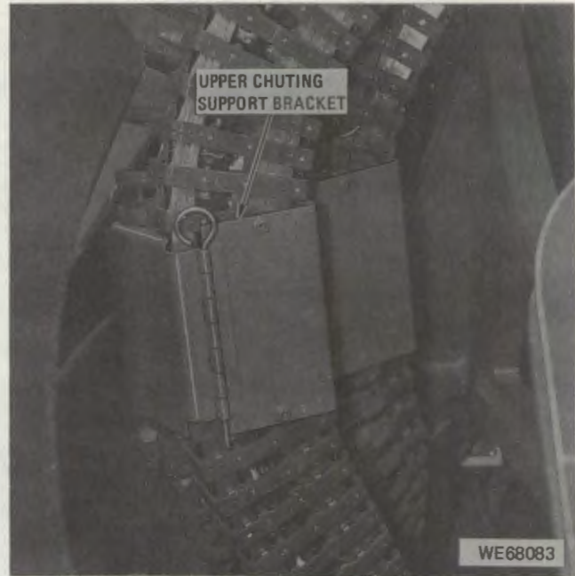
Figure 6-46. XM157 mount, top left view showing location of chuting support brackets (chuting covers removed).
