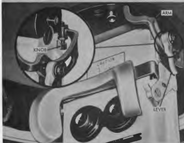
E. Loosen elevation locking lever and set arm adjusting knob so that both ends of elevation arm contact quick release.
