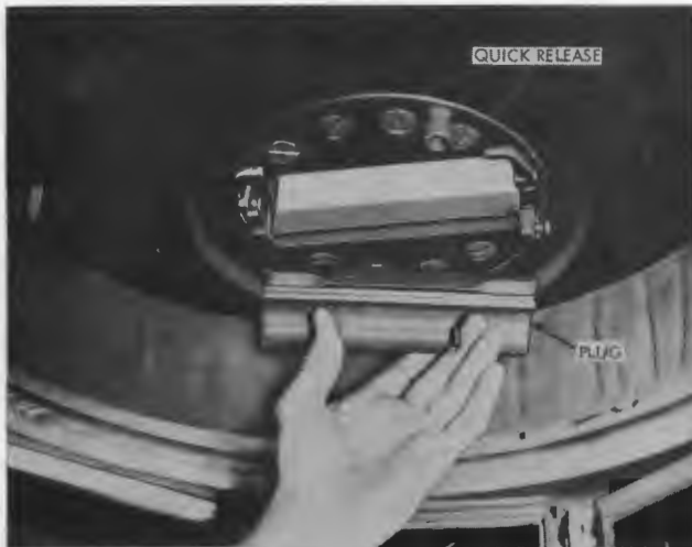
A. Compress quick release, push upward, tilt slightly and bring plug down through hatch cover.
