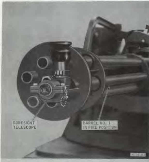
Figure 2-61. Boresight telescope - installed in cannon.
