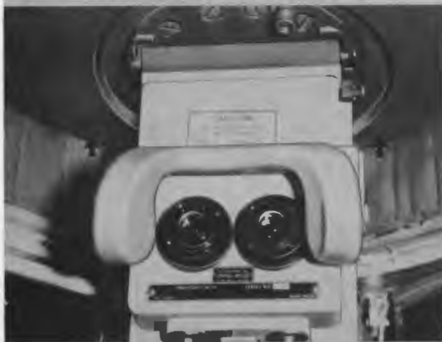
C. Carefully insert periscope and push upward.
