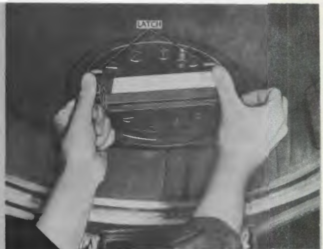
B. Push both periscope latches upward.
