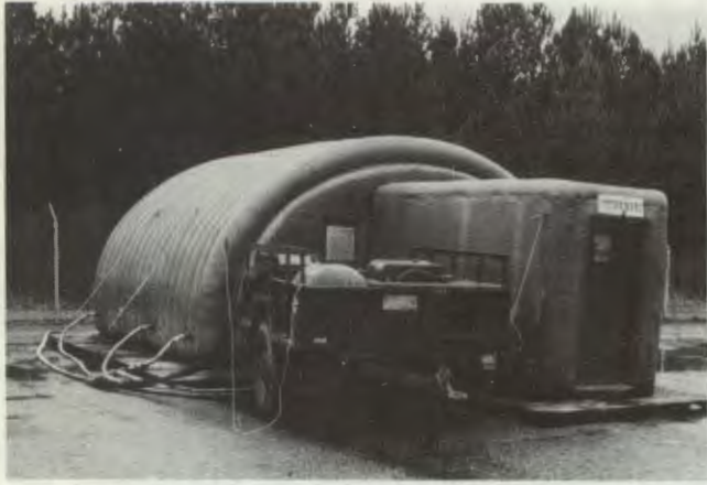
Figure 14-3. XM51 chemical-biological collective protection shelter.
