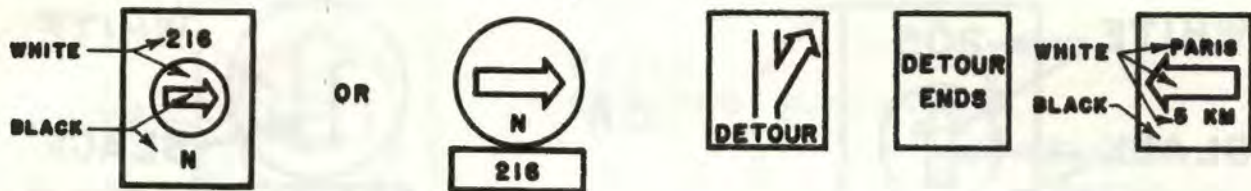
NORTH GOING TRAFFIC TURN RIGHT
