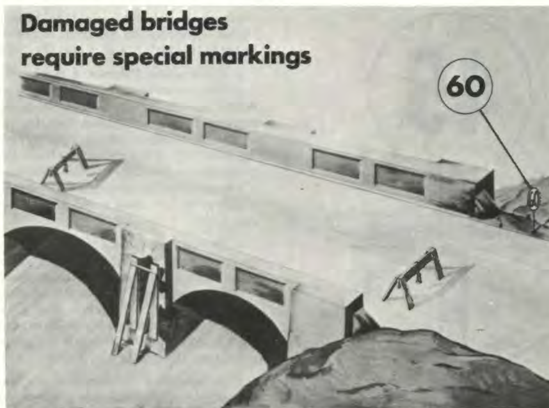
Figure 2-51. Example of posting a damaged bridge.
