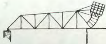
ROLLING LIFT TYPE BASCULE BRIDGE
