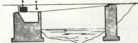
SINGLE LEAF TRUNNION TYPE BASCULE BRIDGE
