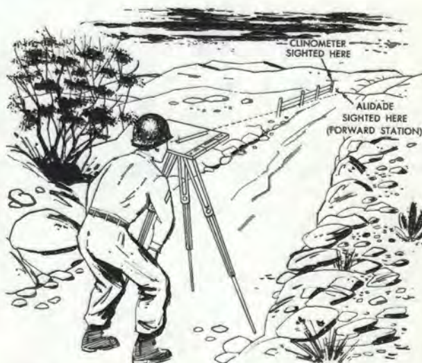
Figure 10-6. Execution of foresight for a traverse.
