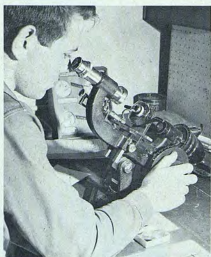
Lenses are shaped and prepared for frames, above right. After being carefully polished, above left, lenses are checked after surfacing procedure is completed.
