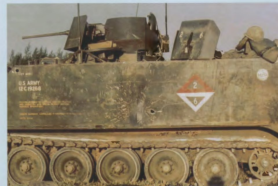
Armored personnel carrier on Operation Russell Beach hit by Vietcong rifle propelled grenade (RPG). (See the hole on the side of the track). (Photo: L.D. Loftis)
