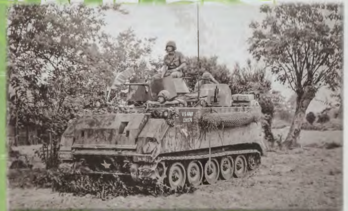
This M-113 in the armored cav carries rolled up fencing on the side of the track, to be used at night as a screen against RPG's.
