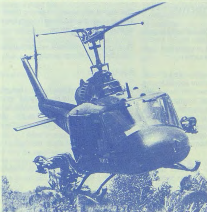
UH-1B of HAL-3 the U.S. Navy "Seawolves", who operated the Huey in the gunship role, beginning in 1966. Note that this B model has been modified with the larger C vertical tail surface. (U.S. Navy)
