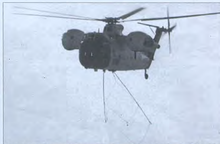
Old 997 flies a test course over White Sands Missile Range, NM, with aluminum poles stretched in a V-shape below her fuselage and hooks ready to catch a drogue chute.
