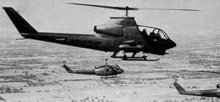
A HueyCobra gunship introduced in October 1967 flies alongside an older UH-1D. The chin turret is directed toward its target by the pilot turning his head. Photo by 1st Aviation Brigade-IO.
