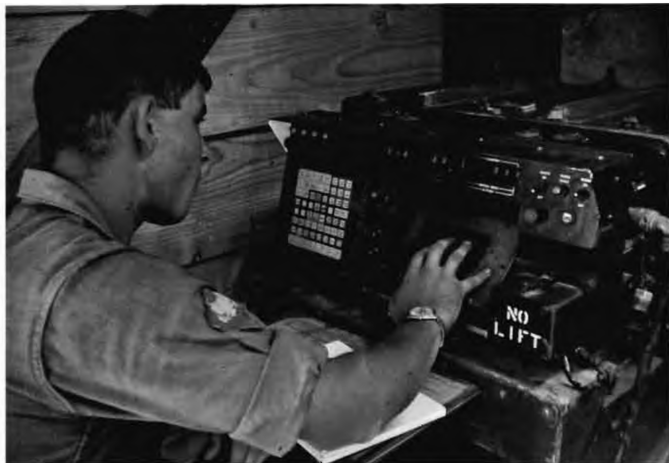
FADAC can control the simultaneous firing of two different weapons. Here is a fire mission being completed by a 175 mm gun and an 8" howitzer from the 7th Battalion, 8th Artillery. The computer can also store data on 88 different targets and control the firing of five different batteries.
