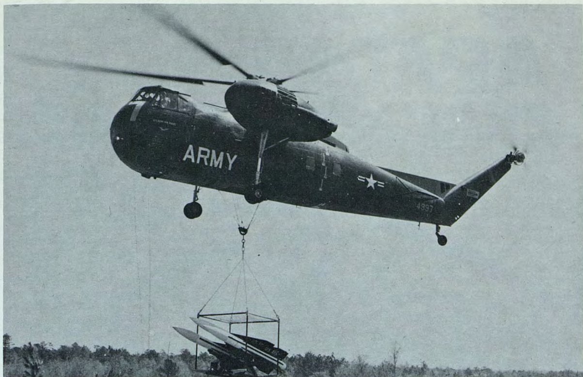
above: The CH-37 shown here lifting the Hawk missile was the Army's first heavy lift helicopter
