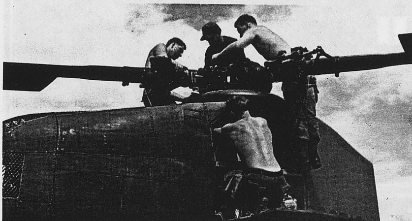
A team of "Shrimp Boat" mechanics removes the rotor blades from their CH-47 Chinook.
