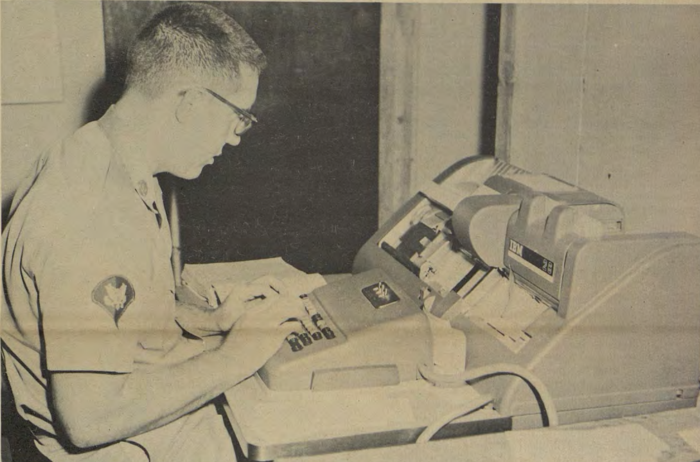
CARD PUNCH - Sp4 Hayes E. Covert, operates an IBM Printing Card Punch machine which punches the individual pay data on a multi-data card.
