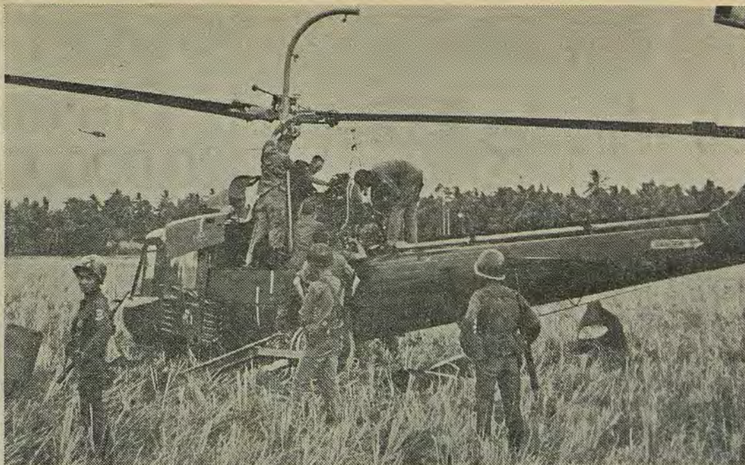
NEW ENGINE ALMOST IN —Service platoon members of the 121st Aviation Company near completion of a new for old engine swap in a Huey. The gunship had a functioning power plant after only 40 minutes, usually a two-hour job.
