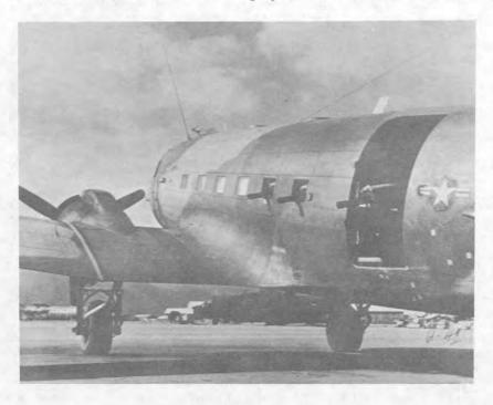
The improved gunship combines detection and destruction in a single, self-contained night attack system. It has proven to be an extremely effective weapon for both interdiction and close air support missions. The first generation AC-47 assets in South Vietnam were turned over to the VNAF in 1969 after the follow-on AC-119's and AC-130's were
