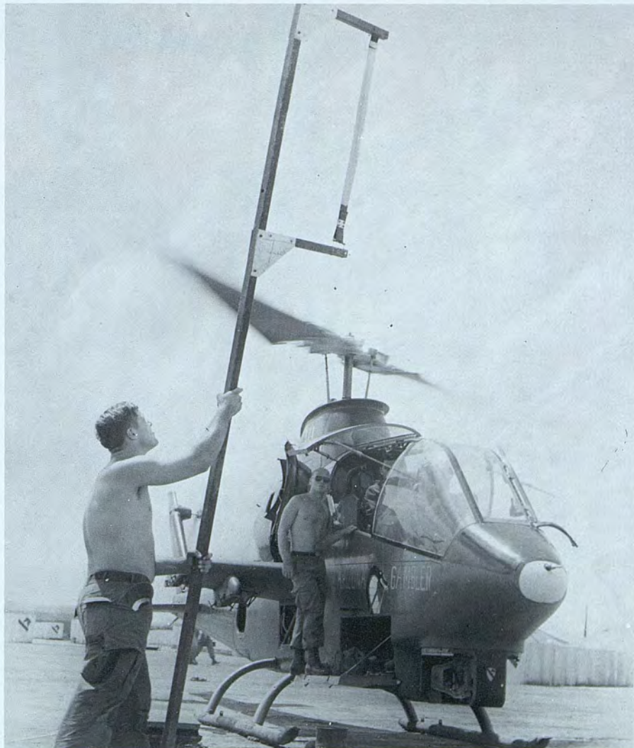
Precision is standard procedure. This new rotor blade must strike the ribbon at exactly the same point before it's A-OK.
