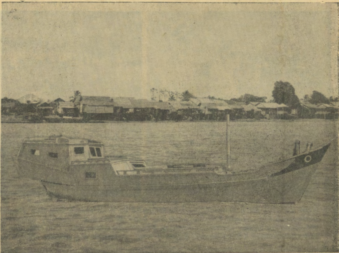
MOTORIZED JUNK — A typical command junk has marine engine for power, can cruise as fast as 15 knots with its 225 horsepower diesel engine. Some motorized junks, unlike one pictured here, also have sails to supple- ment engine.
