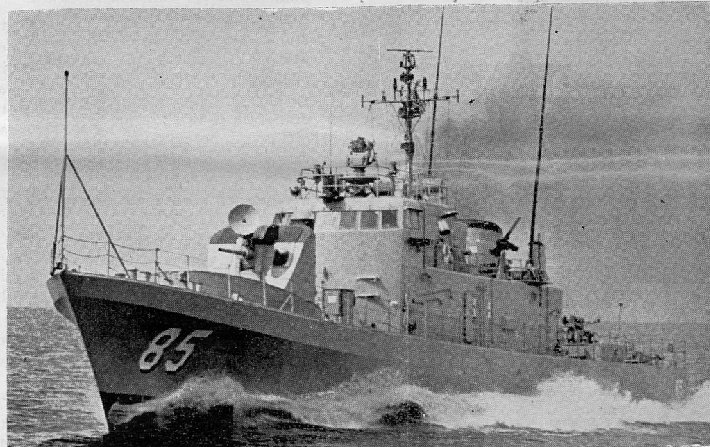
40 KNOTS — The USS Gallup knives through the quiet South China Sea along the coast of South Vietnam on an Operation Market Time patrol. Gallup's 13,500-horsepower turbojet engine is capable of accelerating the ship from 0 to 40 knots in less than 60 seconds.
