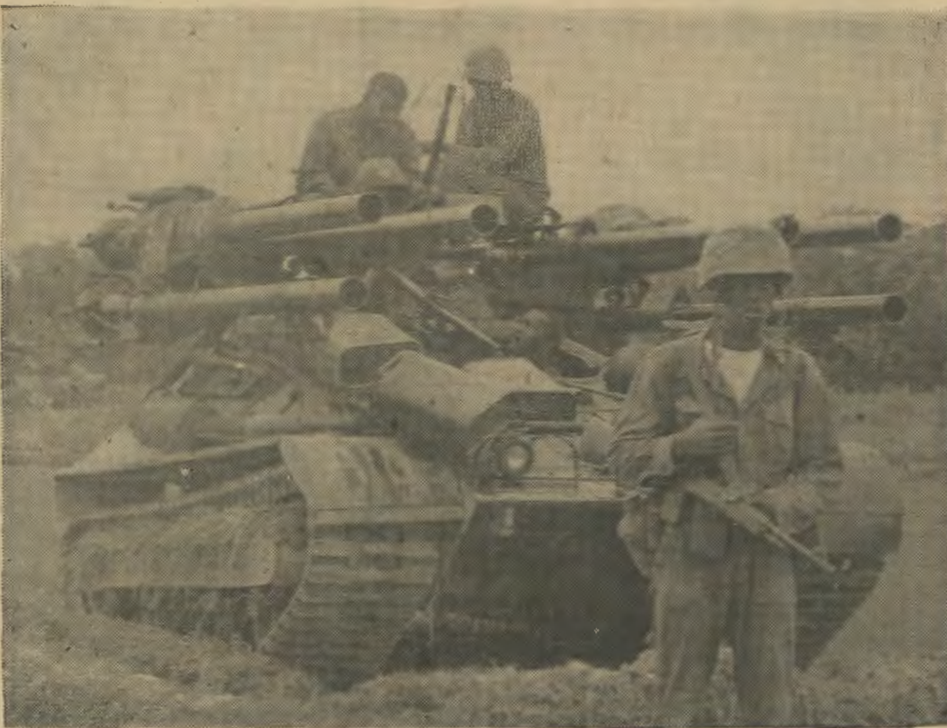
THE THING — A Marine Corps Ontos, which means 'The Thing' in Greek, moves across sodden rice paddies in search of Viet Cong. Its six 106mm recoilless rifles have taught the VC to fear the squat, tracked weapons. (Photo by LCpl. D. D. Kinton, USMC)
