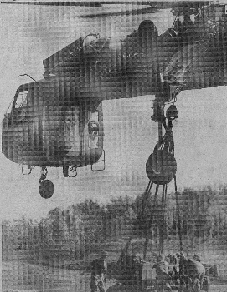
A Flying Crane drops a bulldozer to 8th Engineers for quick clearing operations at the site of air strip construction at Bu Dop.
