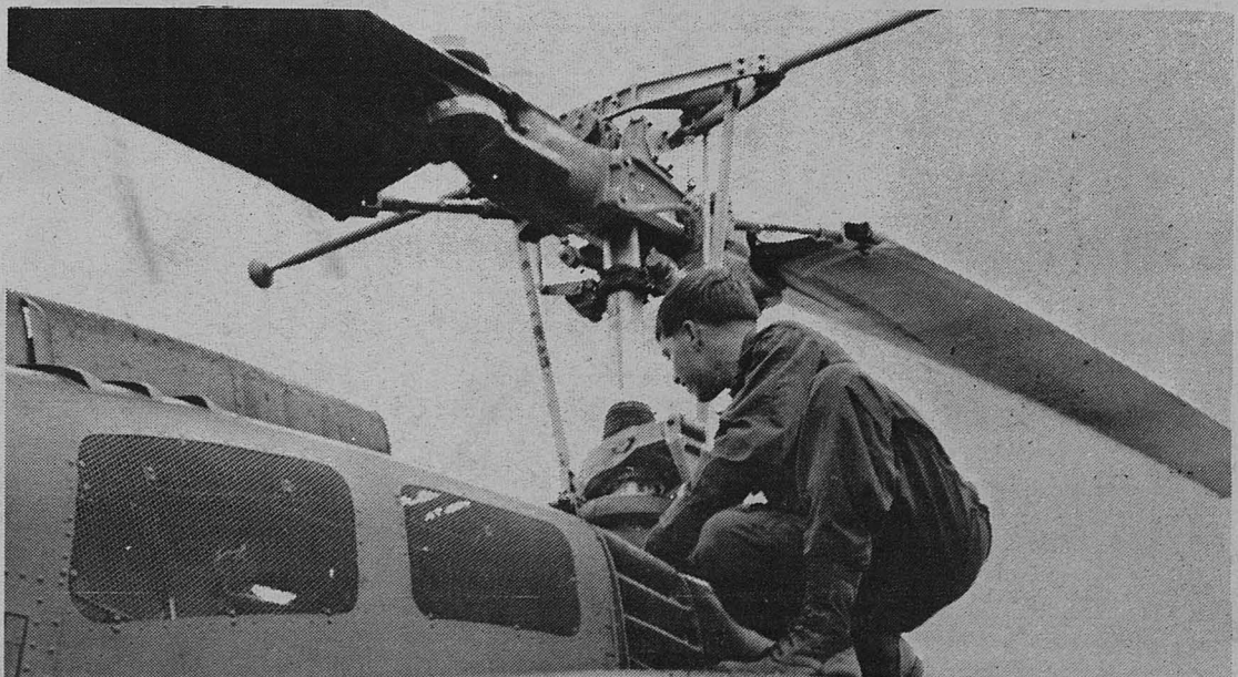
Warrant Officer Olson performs a pre-flight check on the main rotor. This is only one of the basic steps in the helicopter test pilot's checklist.
