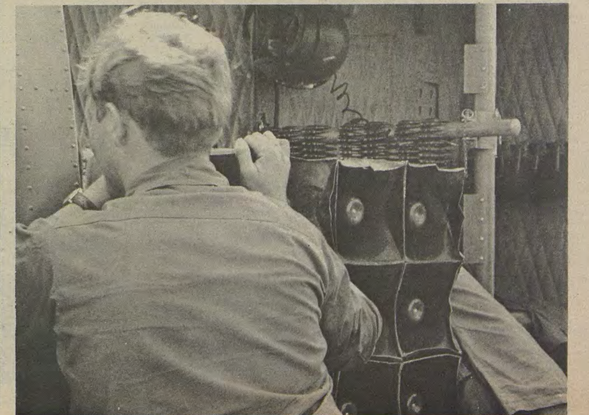
(U.S. ARMY PHOTO BY SFC Peter De Gard) The broadcast speaker assembly is mounted on the side of a Huey slick prior to takeoff.
