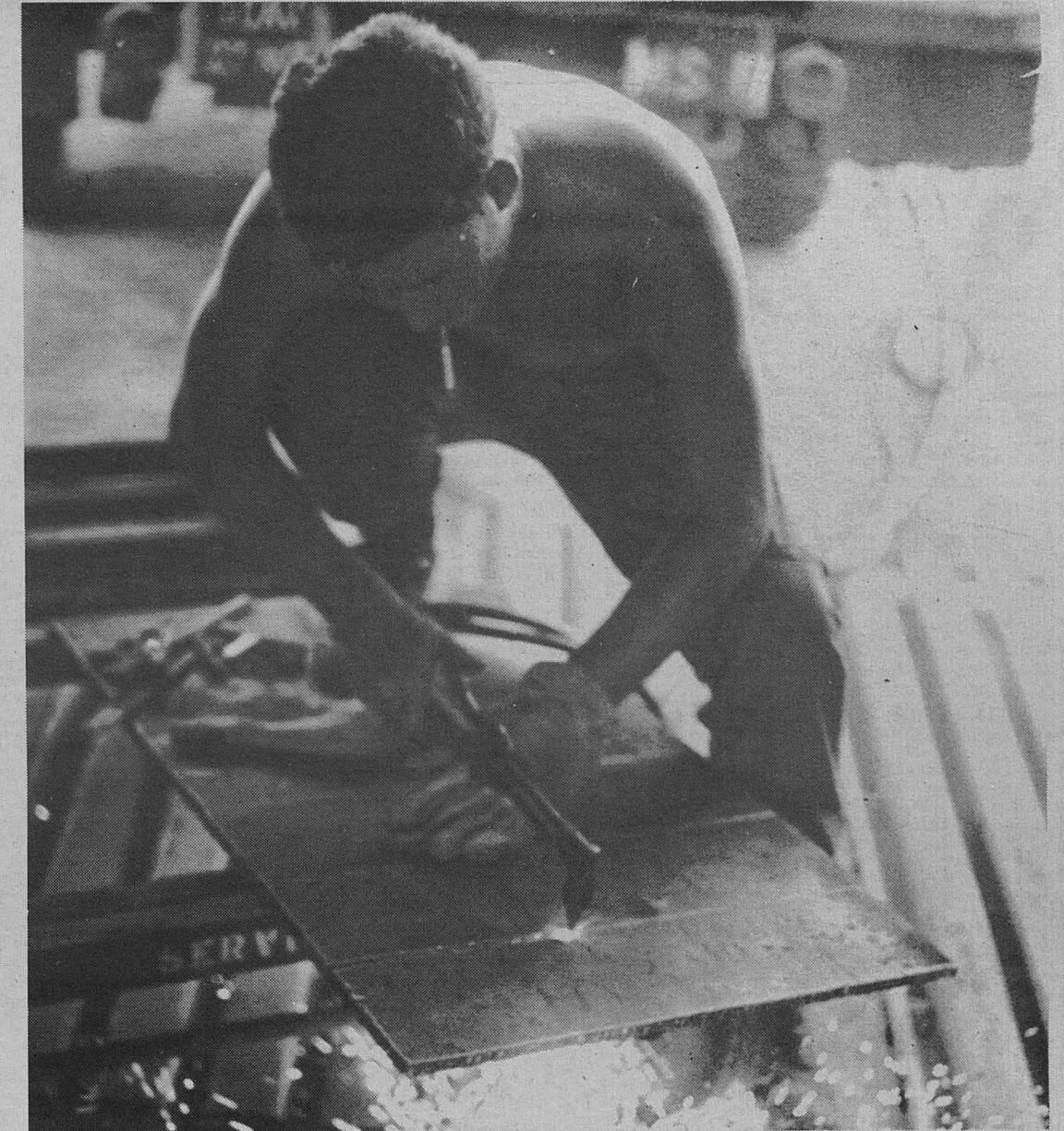
Welder Specialist Four Bruce Sexton uses an acetylene torch to cut through sheet metal.
