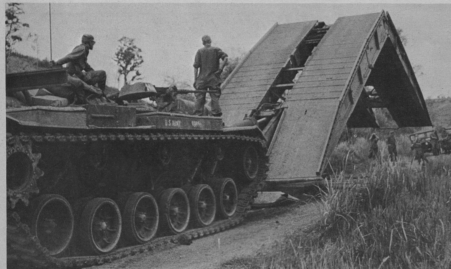
The Armored Vehicle Launch Bridge swings into action from its resting place atop the track. The 40-foot portable bridge was used in crossing deeper streams that the convoy was unable to ford.
