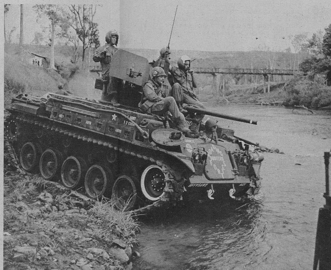
Equipped with twin 40mm cannons, the Duster inches its way into the Song Be River. Rivers proved no obstacle for the tracked convoy as the self propelled guns tread water in their journey to their new firebase.
