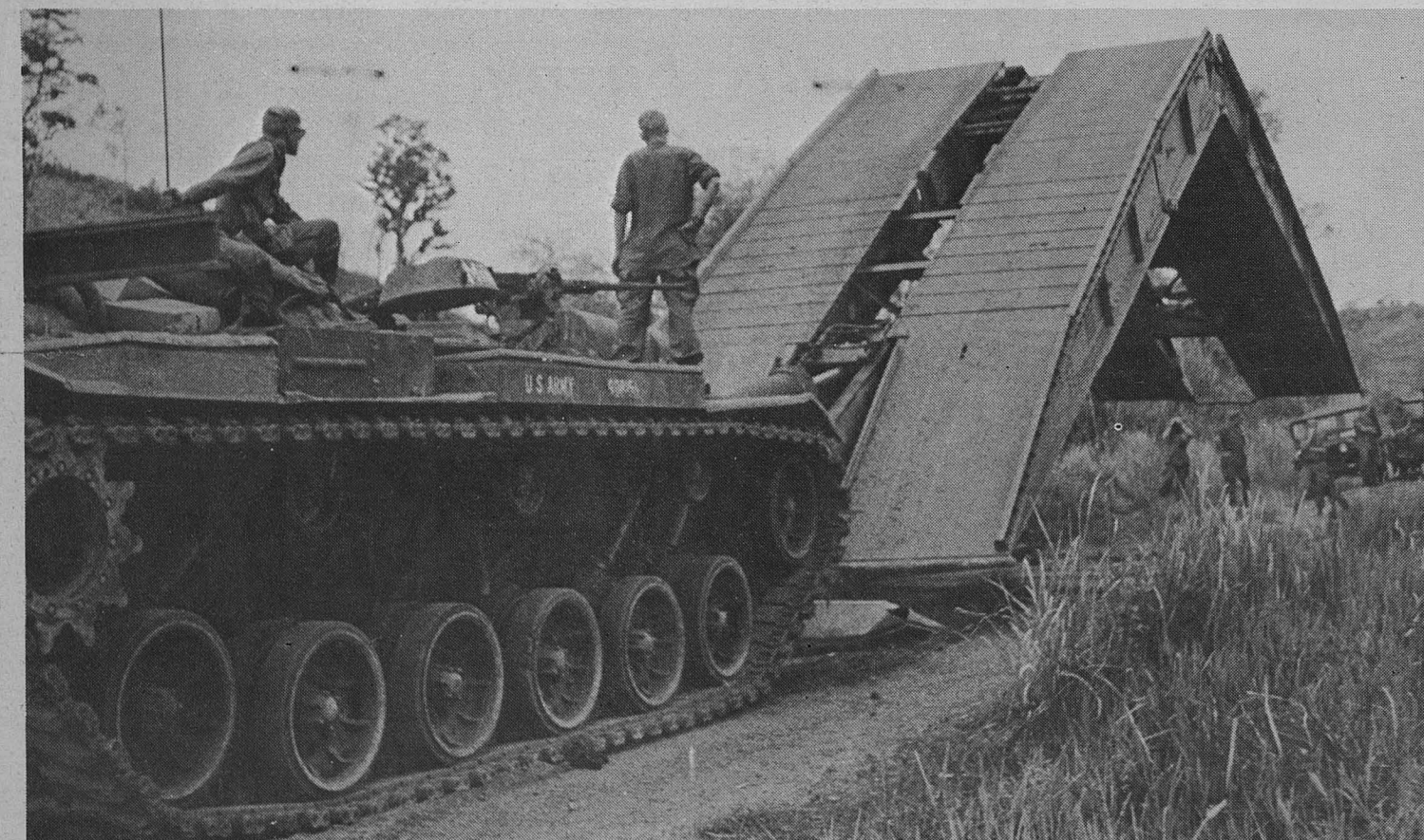
The Armored Vehicle Launch Bridge swings into action from its resting place atop the track. The 40-foot portable bridge was used in crossing deeper streams that the convoy was unable to ford.
