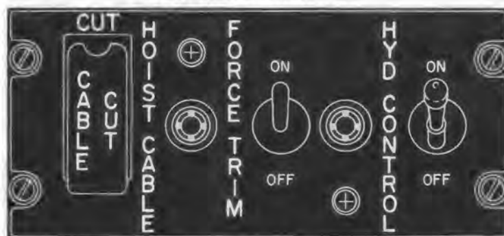
HYDRAULIC, FORCE TRIM, AND HOIST POWER CONTROL PANEL
