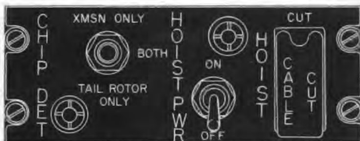
CHIP DETECTOR AND HOIST POWER CONTROL PANEL
