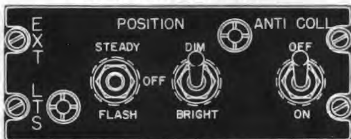
EXTERNAL LIGHTS CONTROL PANEL
