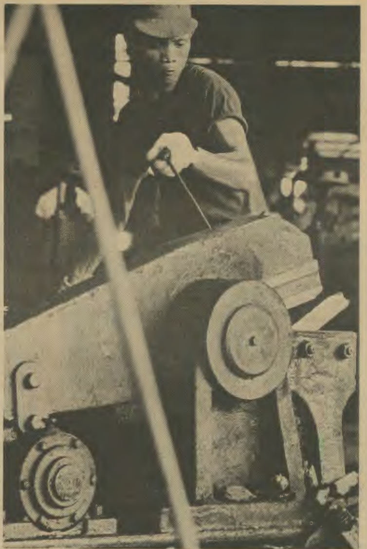
A hydraulic clipper removes inferior steel from end of each ingot.
