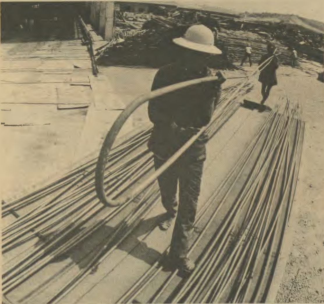
Finished product -- steel rods for strengthening concrete -- is ready for loading on trucks bound for Saigon.
