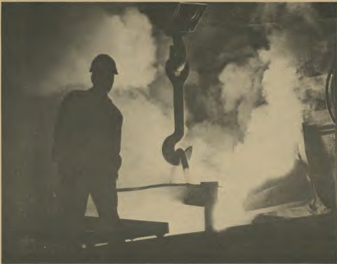
A worker guides a giant bucket as it dips molten steel from a pit beneath furnace.
