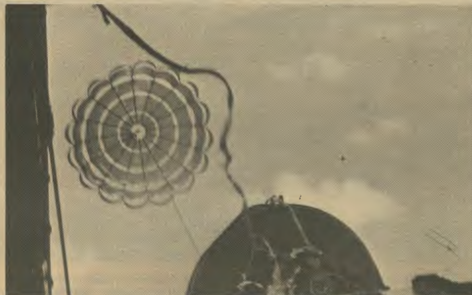
BOMB AWAY -- A billowing extractor chute pulls the high-yield, low fragmentation bomb from the cargo deck of the C-130.
