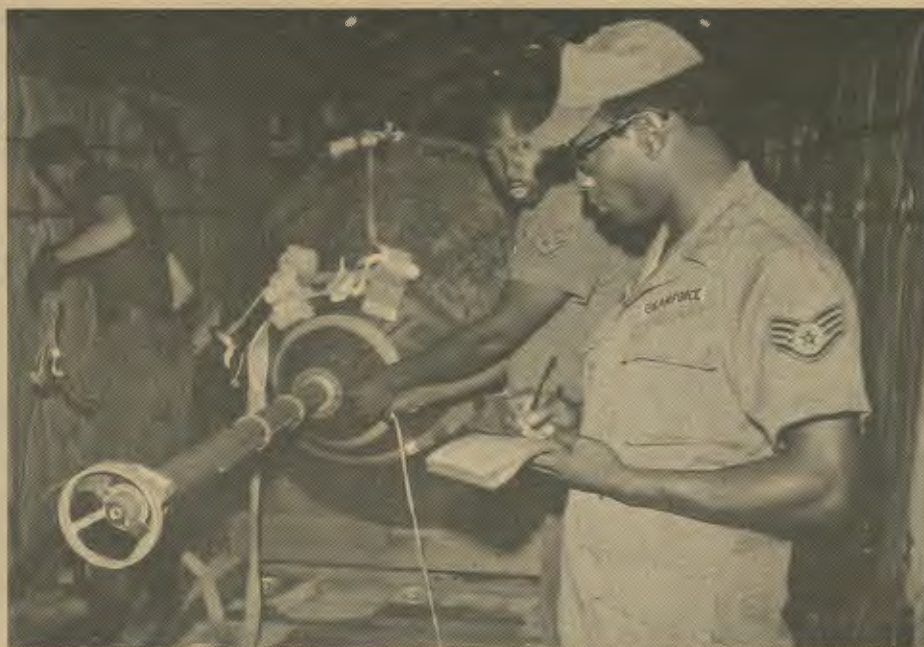
THREE FEET GOES A LONG WAY -- Munitions specialist of the 483rd Munitions Maintenance Sqdn. install a 3-foot long fuse that will detonate the bomb above ground to maximize lateral blast effects and avoid causing a deep crater.
