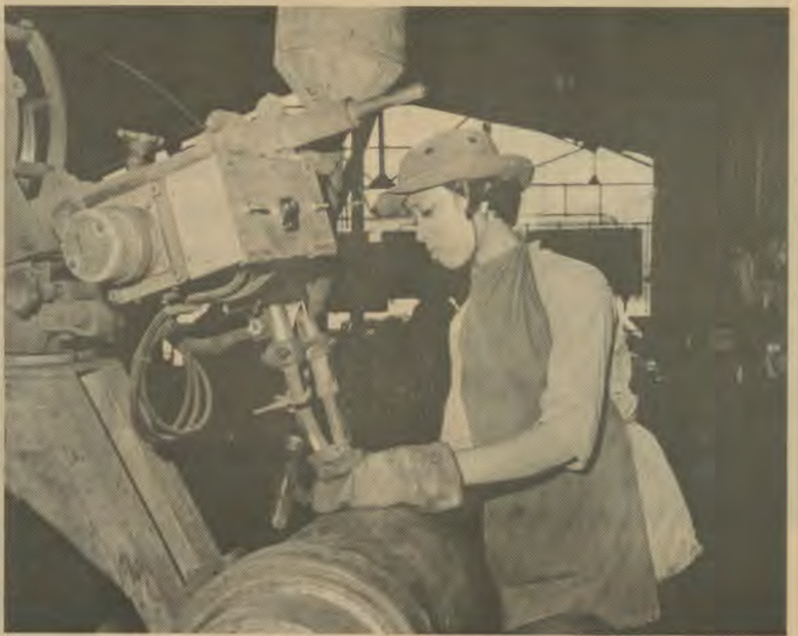
A Vietnamese girl operates a seam welder used in the fabrication of gas cylinders.
