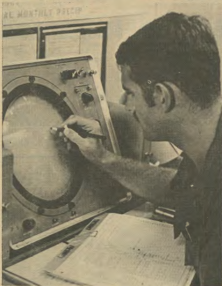
THUNDERSTORMS - Air Force Captain Bruce M. Nagle plots the movement of a thunderstorm which threatens to interfere with local flying patterns on a small radar unit.
