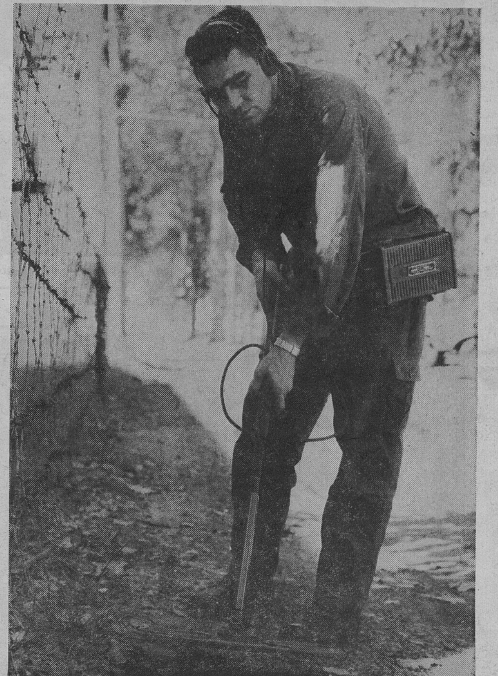
An EOD man uses a MK-10 Ordnance Detector and Locator in search for land mines
