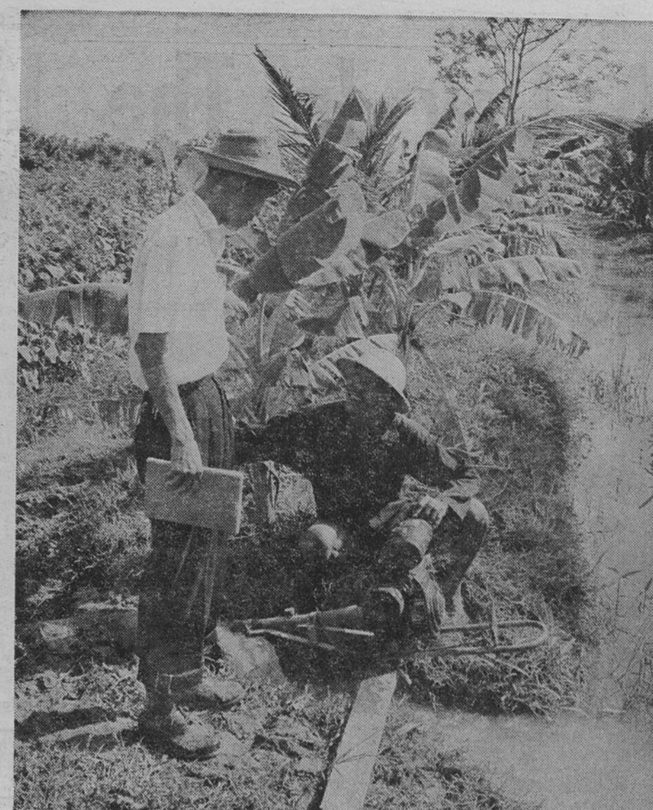
The converted outboard motor draws water into an irrigation ditch.
