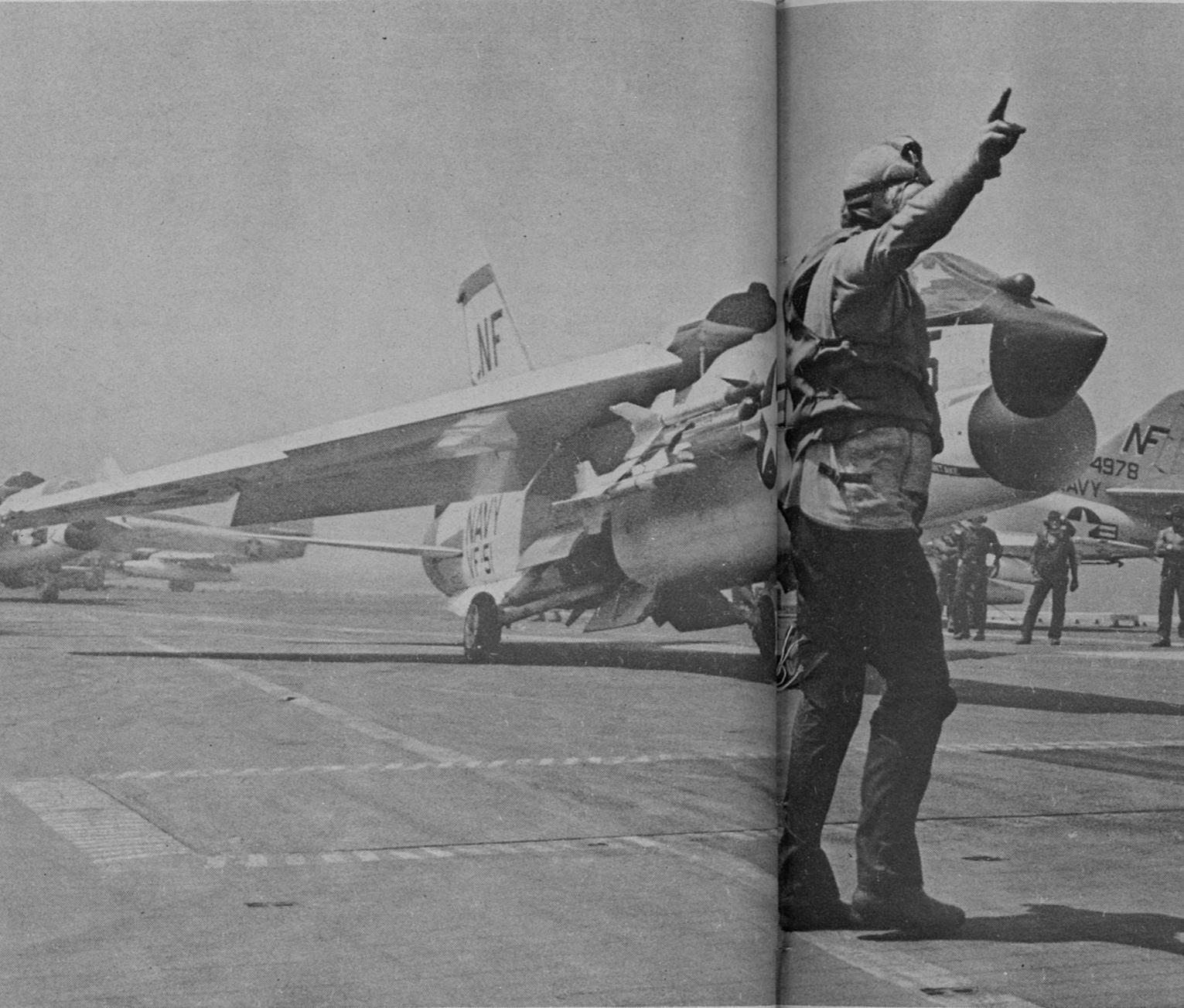
A Plane Director gives commands to the pilot of an F-8 "Crusader" as the pilot approaches the catapult before being launched into attack.
