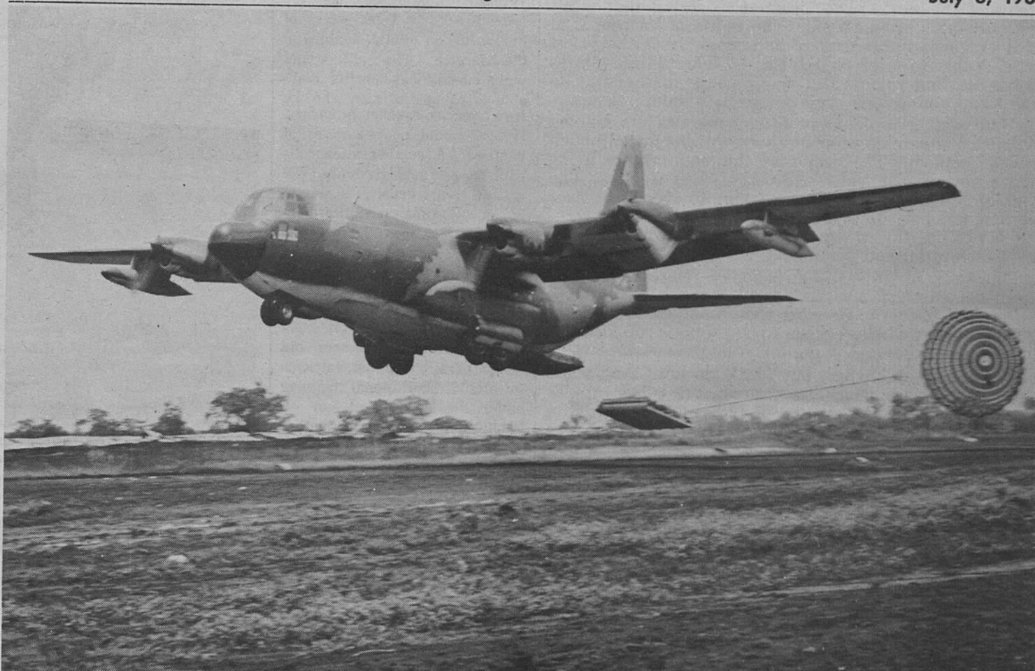
LAPES DROP—An Air Force C-130 Hercules makes a Low Altitude Parachute Extraction System (LAPES) drop of supplies to an Army outpost. (USAF PHOTO)
