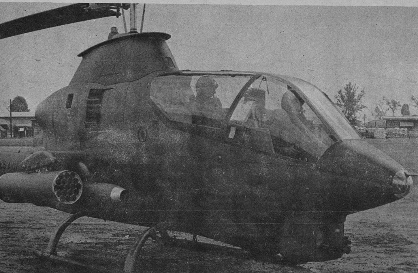
The Cobra is a flying arsenal with its 38 rockets, two fixed mini-guns, turret mounted mini-gun and 40 mm grenade launcher.
