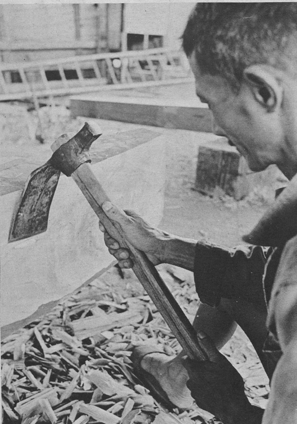
Using a cutting tool indigenous to the Orient, a craftsman planes the keel.
