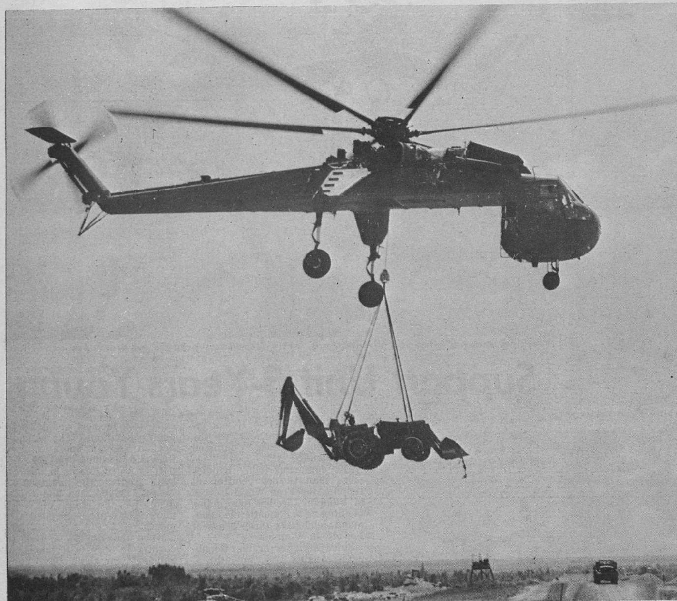
Wasting no time a "skycrane" carries a "backhoe" tractor to where a new 101st fire support base is being built.
