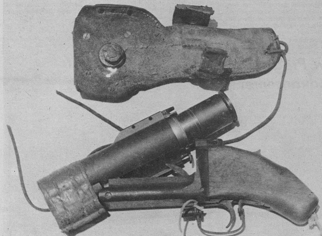
BIG GUN —This big-bore weapon was captured by 3rd Marine Division Leathernecks during an engagement with the North Vietnamese Army near Dong Ha. The "big gun" has been fashioned from a M-79 grenade launcher and is equipped with a fast-draw spring holster made from a cut down U.S. pistol holster. (USMC PHOTO By: LCpl. Bob Stetson)
