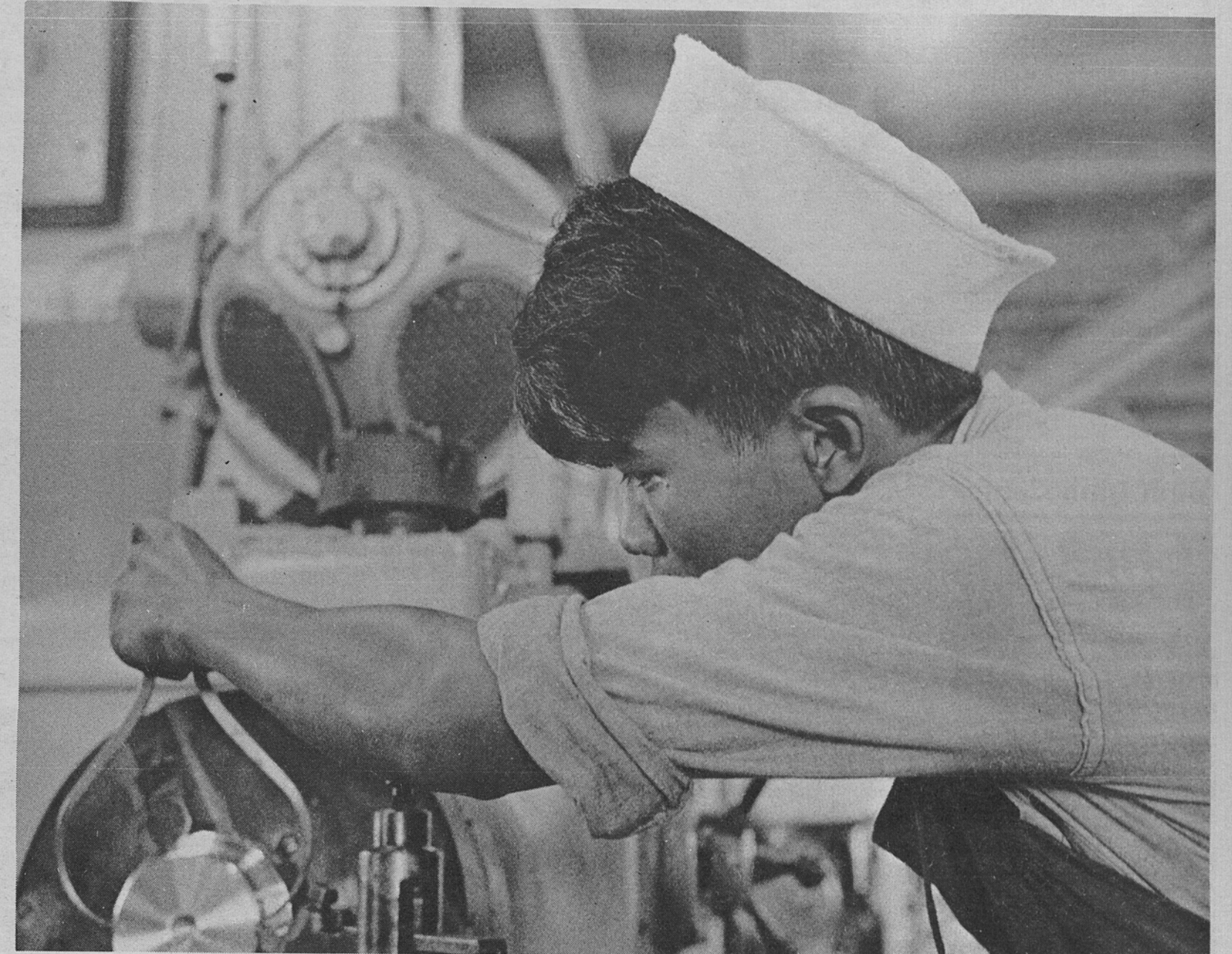
Using the skill he learned from U.S. advisors, a Vietnamese sailor checks the tolerance of a replacement part he is turning on the lathe.
