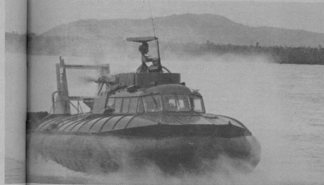
Hovering cushion of air, the air cushion vehicle can travel over land or water with equal ease.
