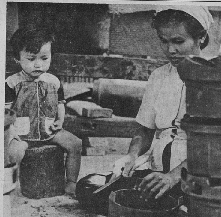
Before painting, rough edges of stove must be filed down.
