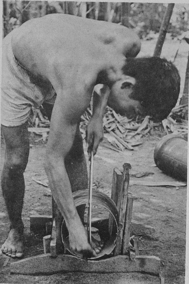
Worker starts to cut into top of stove to create legs, grill.
