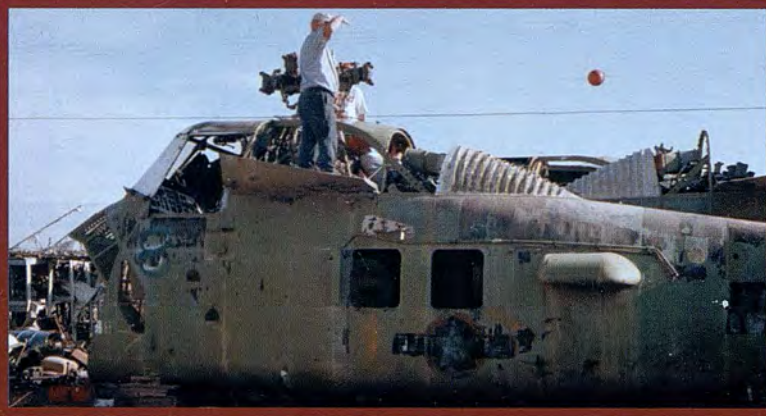
A.C. Daniel & Ron Hatton getting the aircraft ready to remove the transmission/rotor head assembly from the air-frame.
