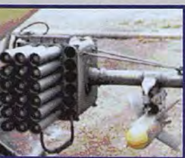
Maxwell System showing three banks (18 rockets) and one AGM-22B
