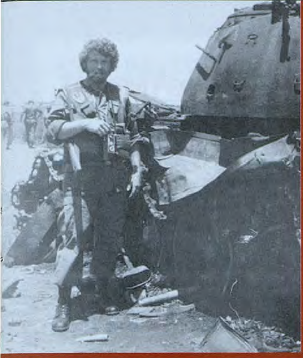
Kenneth Blum was one of the TOW technical representatives from Hughes Aircraft that went over to RVN with us. Here he is pictured in front of a Russian-made T-54 tank destroyed by the TOW missile system. Visible is the hole made by the shaped-charge on the side of the turret. Also visible at his feet is the rocket motor from the TOW Missile.
