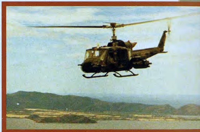
Camouflaged UH-1B with XM-26 TOW armament subsystem.
