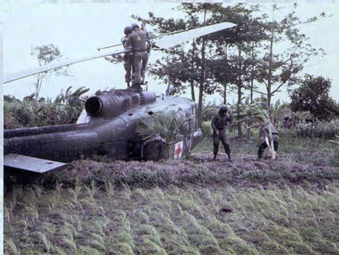
56th Transportation Company recovery crew rigging Dust-Off for extraction by CH-47 Chinook, IV Corps area, September, 1967.
