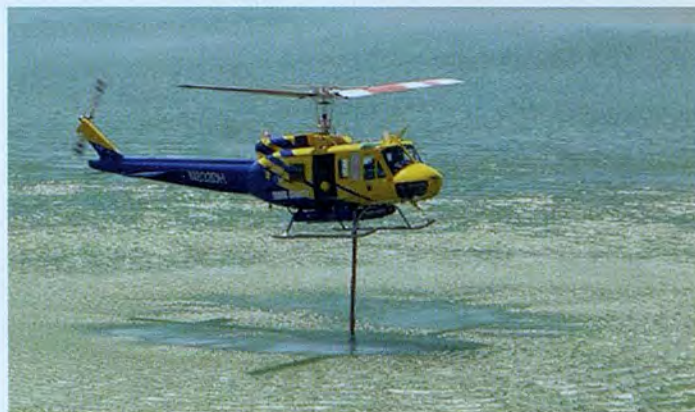
659 can fill up her 325 gallon tank from almost any fresh water source in 40 seconds using their on-board snorkel. Willy assures me they try to stay away from private swimming pools.
