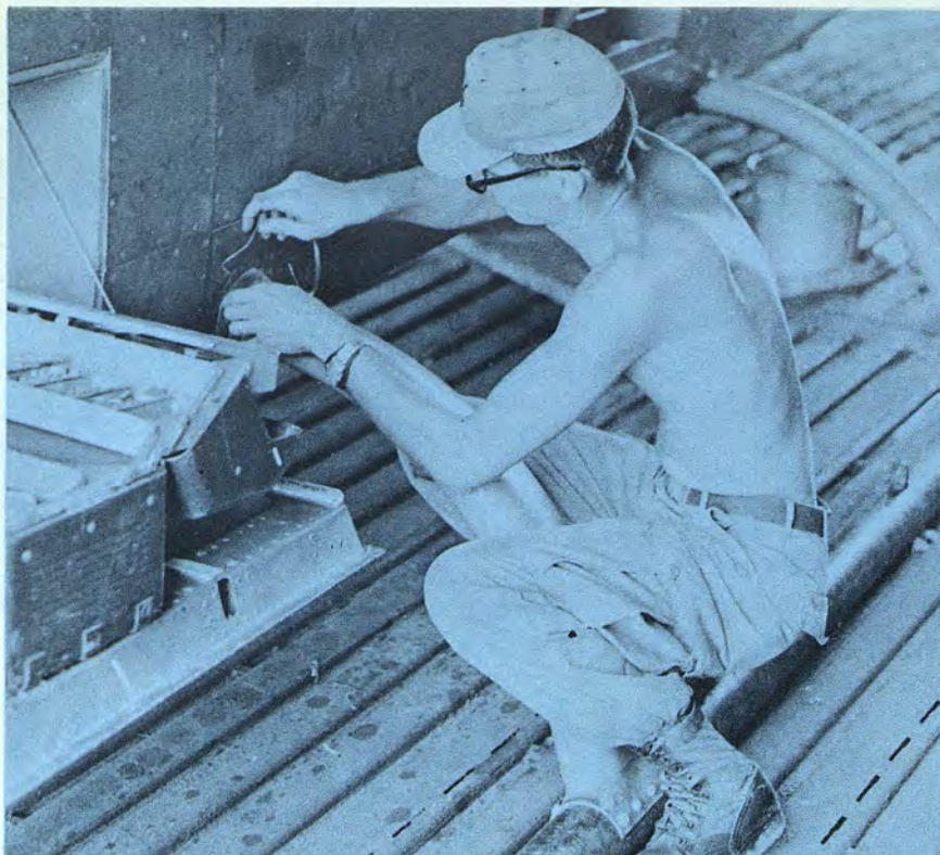
Severe vibrations in rotary wing aircraft necessitate careful assembly procedures. Specialist Five Michael E. Shelbert safety wires the seal on a Cobra cross-tube so that it can't loosen because of vibrations.
