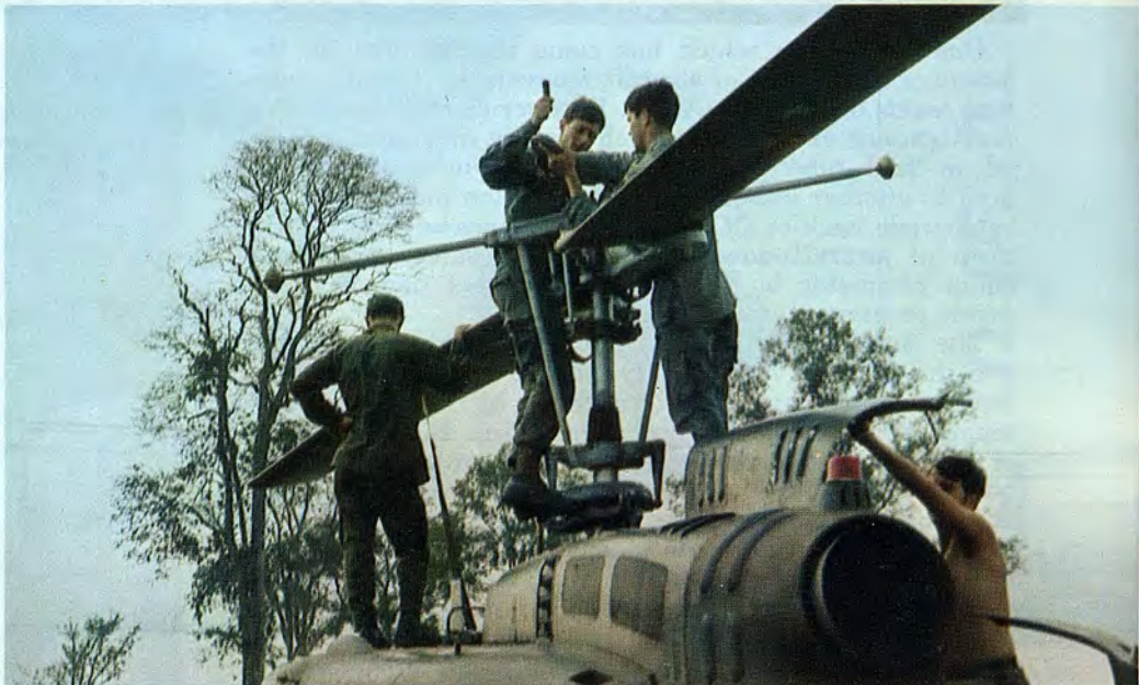
On field recovery missions, the rigging team is often confronted with difficult situations. The aircraft pictured at the top of the page had to be lifted out of this wooded area by a Chinook and set down in a clear field so that the main rotor blades could be secured fore and aft.
