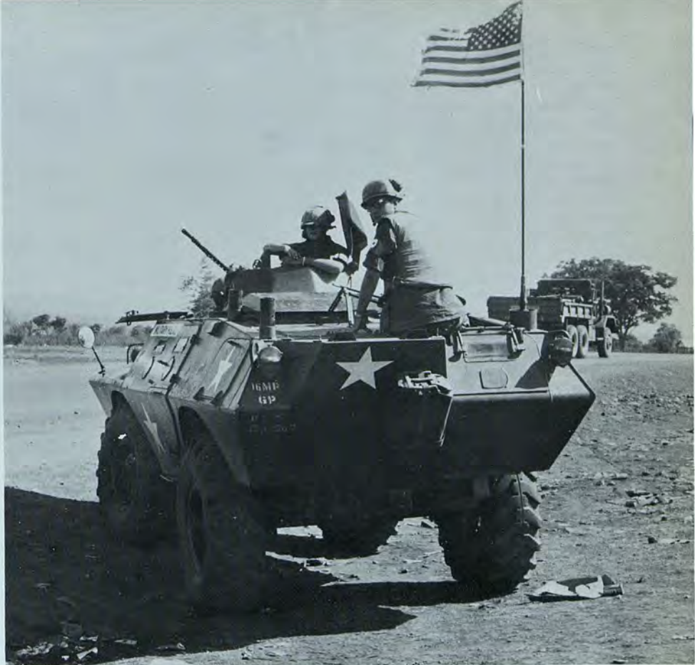
A 560th MP Company V-100 prepares to leave checkpoint 88 near Pleiku on a convoy run to An Khe. The experimental armored commando car, equipped with twin M73 and M60 machineguns, can reach a speed of 70 miles an hour.
