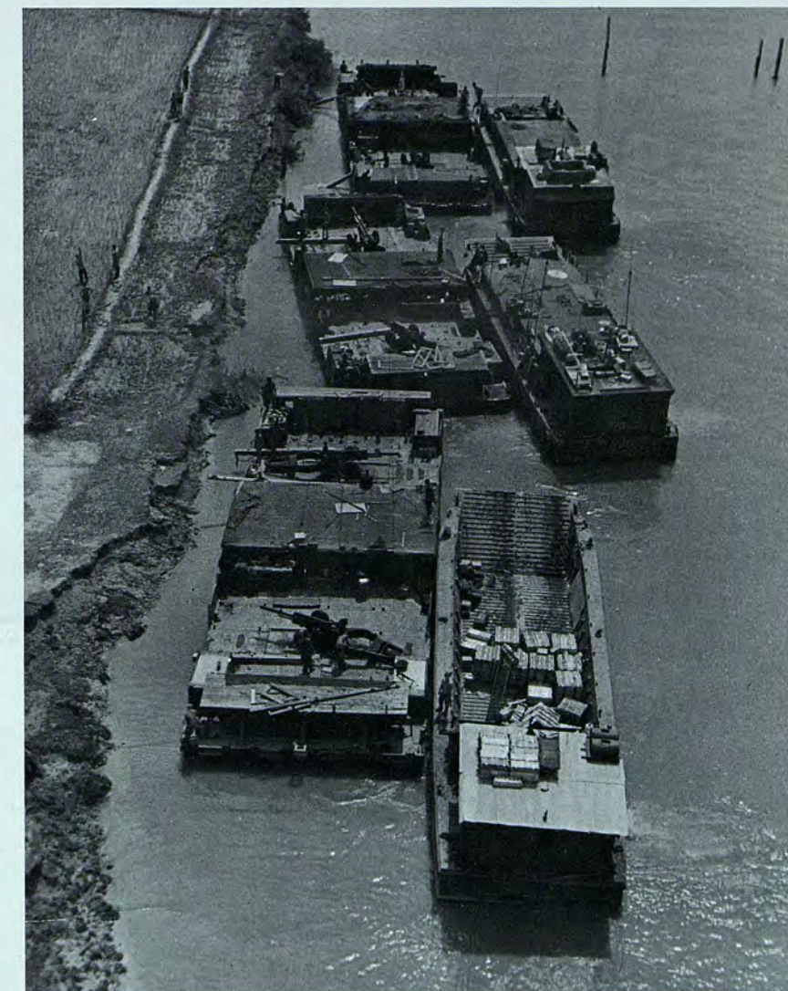
Quick movement of artillery has been aided by floating platforms that allow the 3d Battalion, 34th Artillery to displace easily in the river-laced Delta. In a matter of minutes, the platforms can move out to a new position.
