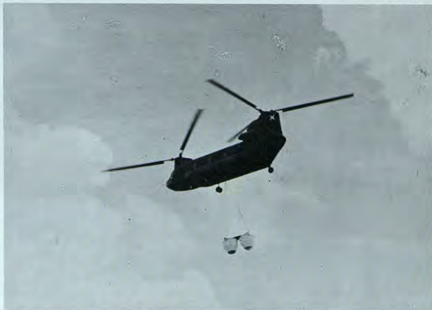
Attached underneath the CH-47A (Chinook), each bucket carries 450-gallons of water
