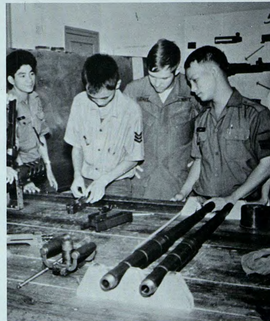
Field-stripping a .50 caliber machinegun
