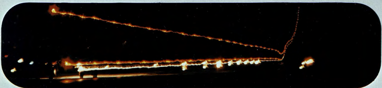
A time exposure of a fixed wing takeoff shows a red dot-dash pattern from spinning fuselage and wingtip lights.
